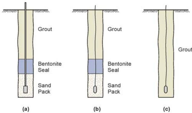
Figure 1(a). Traditional standpipe piezometer with sand pack.
