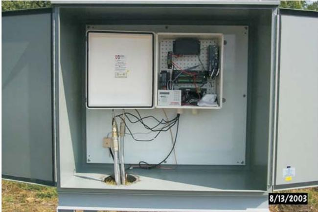
Figure 1. TDR data acquisition system. Four coaxial cables are connected to the multiplexer inside the smaller cabinet. The datalogger, TDR unit, external storage module, phone modem, and auto-dialer are also in the smaller cabinet.
